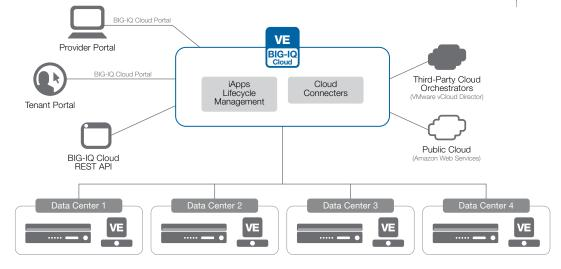
F5 BIG-IQ Cloud components integrate and collaborate to provide consistent, cross-environment management of application network services.
