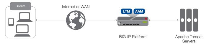
**Figure 1:** Using the BIG-IP system as a reverse proxy
