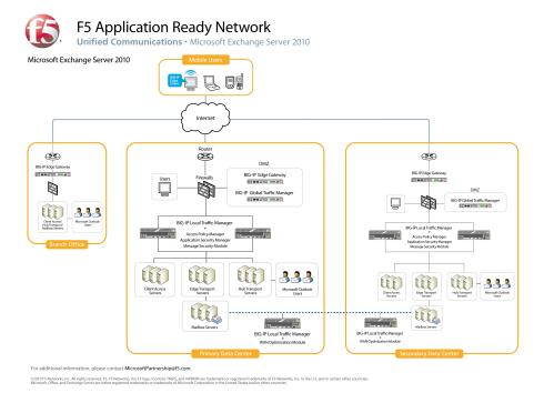
Deployment architecture for complete F5 solution for Exchange Server 2010
