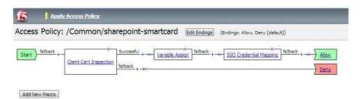
Manually configuring the BIG-IP Advanced Firewall Module to secure your SharePoint deployment
