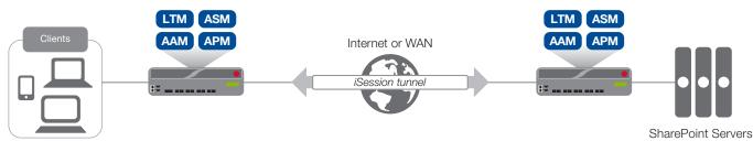
Figure 2: Using an iSession tunnel to secure and optimize traffic between two BIG-IP systems
