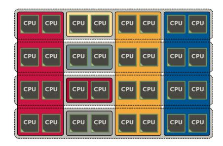
When vCMP is deployed on a multi-blade VIPRION system, administrators can configure the vCMP instances of ADCs in multiple ways. The instances may exist on single blades, or they may span multiple blades. In addition, since VIPRION chassis allow new blades to be added on the fly, vCMP instances can be configured to automatically expand across the new blade resources without interruption. The primary benefits of vCMP are:
